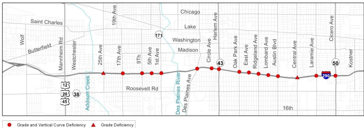
Figure 1-14 - Existing Crossroad Vertical Geometry Deficiencies
